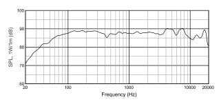
Measured on-axis with distance referenced to 1 meter at 1 watt, half-space (126W)
